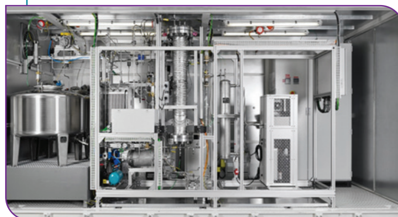
The pre-commercial hydrogenation plant procured in collaboration with Framatome GmbH.
