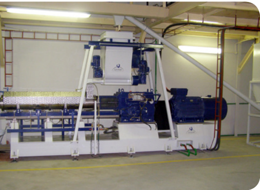
The TX80 twin-screw food extruder in FeedPro's dog food plant.
