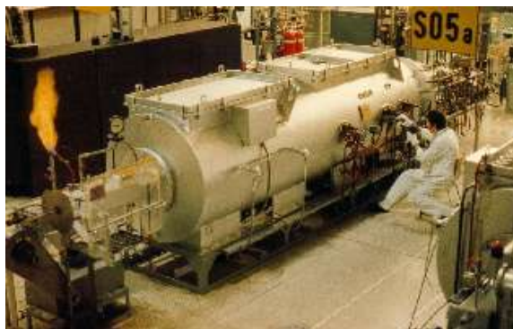
Sintering Furnace for UO 2 Pellets
